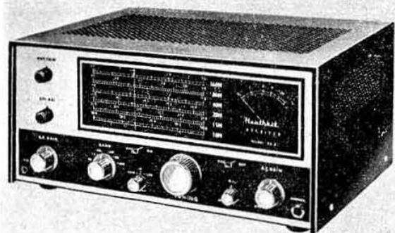
The Heathkit Model RA-1 amateur bands receiver. The cabinet is finished in silver and green. The panel controls (reading from the top left) are aerial trimmer, calibration adjustment, r.f. gain, band-switch, b.f.o. on/off, sideband selection switch, main tuning, a.v.c. on/off, noise limiter and a.f. gain. The phones jack is at the bottom right-hand corner of the front panel.
