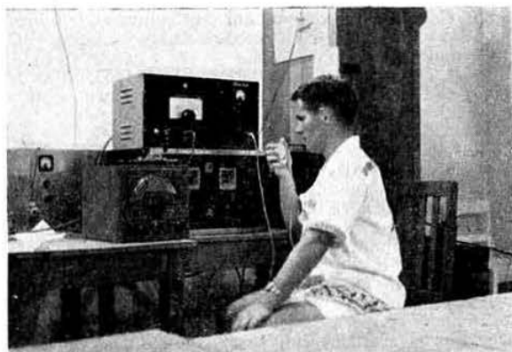
VR2EH in Fiji uses a Panda Cub transmitter and a Hammarlund receiver.
